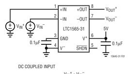
$$V_{IN} (COMMON MODE) = \frac{V_{IN}^+ + V_{IN}^-}{2}$$
