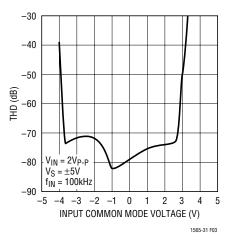
Figure 3. THD vs Common Mode Input Voltage
